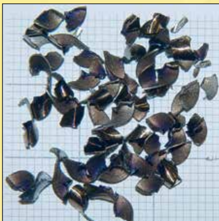
Short, problem-free chips preventing chip congestion and binding of the tool.
