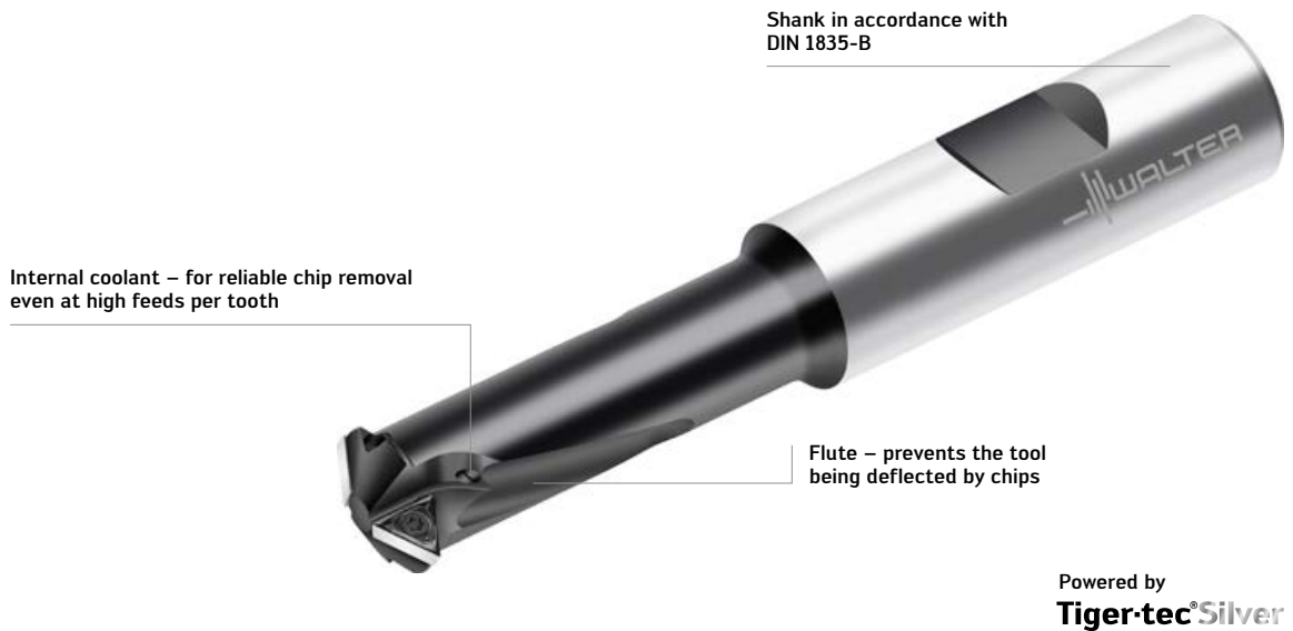
T2711 indexable insert thread milling cutter
